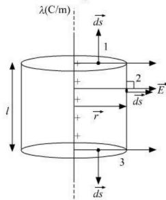
In the diagram we have taken a cylindrical gaussian surface of radius = r and length = l. The net charge enclosed inside the gaussian surface qenclosed =  $\lambda$ l and length = l. By symmetry we can say that the Electric field will be in radially outward direction.
