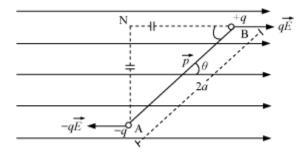
Consider an electric dipole consisting of charges  $\neg q$  and +q and of length 2a placed in a uniform electric field  $\vec{E}$  making an angle  $\theta$  with the electric field.
